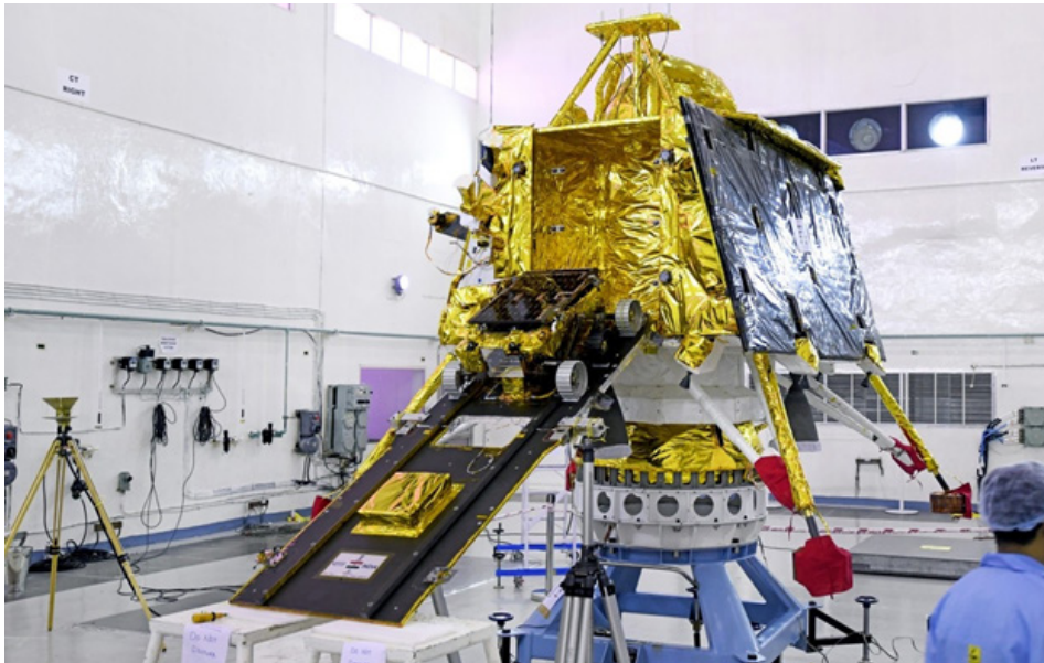
Pragyan Rover mounted on the ramp projecting from out of the sides of vikram lander | Photo: ISRO
